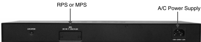
Figure 1-2. Back-Panel Power Connector
